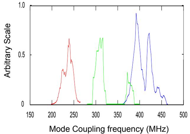
Figure 2. Typical mode-coupling frequency response of an anisotropic leaky-mode modulator, depicting nearly non-overlapping acoustic spectral bands that act exclusively and independently upon red, green, and blue light.
