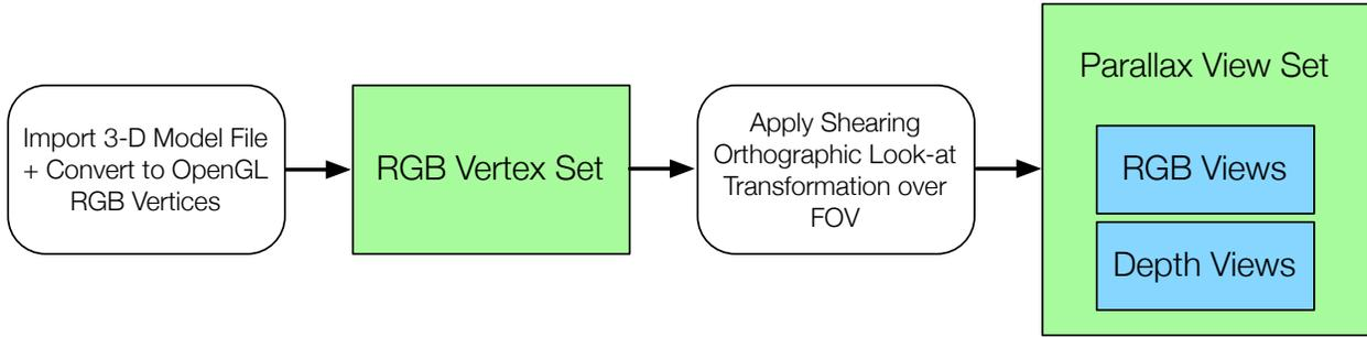
Figure 6. Process flow for generation of orthographic views from 3-D model input in an OpenGL context. 3-D model input is converted to a set of vertices with associated color values, upon which a look-at matrix (corresponding to viewing the scene with a double frustum camera geometry) acts over the desired field of view to generate a set of 16 orthographic RGB views and 16 orthographic depth views.
