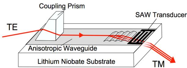
Figure 1. Structure and function of an anisotropic leaky-mode device, implemented as a guided-wave device on a LiNbO<sub>3</sub> substrate.
