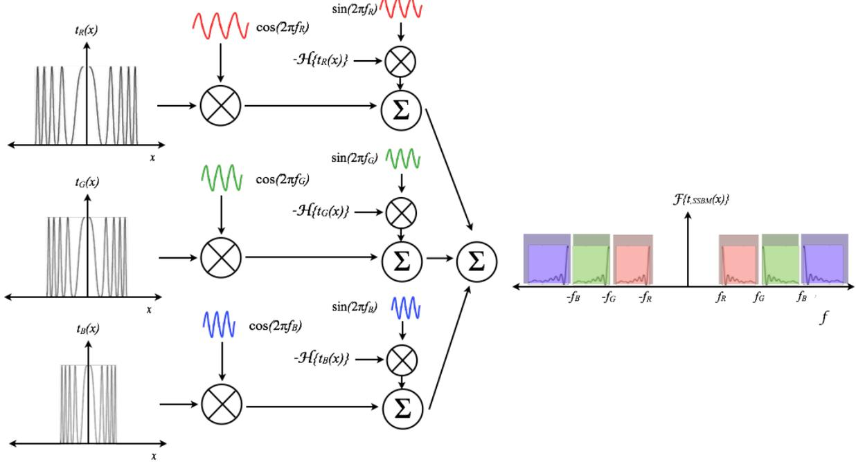
Figure 3. Depiction of single-sideband modulation process and frequency-division multiplexing scheme for generation of appropriate fringe signal for input to Mark IV electronics in the case of a general CGH.
