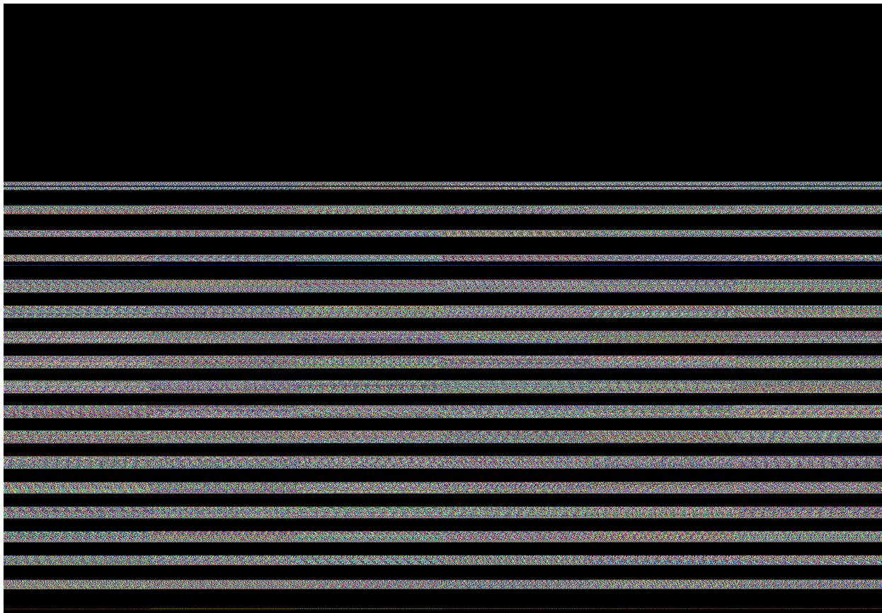
Figure 12. Fringe buffer displayed on the output of one GPU head, containing holographic information for 26 holographic lines for each of three analog channels (corresponding to the nominal red, green, and blue output channels of the GPU).
