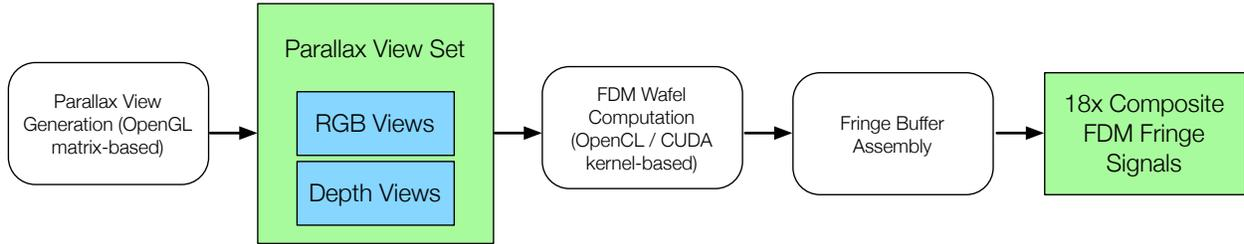
Figure 8. GPU-based pipeline for computation of frequency-division multiplexed fringe signals based on the diffraction-specific coherent panoramagram approach. Orthographic views in RGB and depth are generated in an OpenGL context as used as input for parallel wafel computation, implemented in either CUDA or OpenCL kernels.
