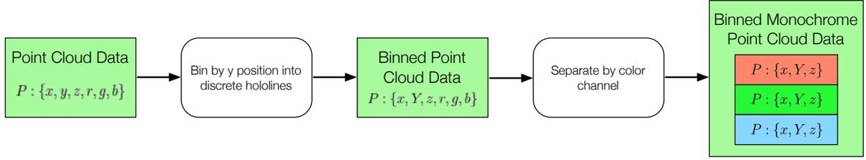
Figure 4. Process flow for generation of monochromatic, hololine-specific point cloud data from full-color, three-dimensional point cloud data. Beginning from 3-space coordinates and RGB information per point, points are binned into 468 discrete y-values. All points in each bin are then separated by color channel into constituent monochromatic points.
